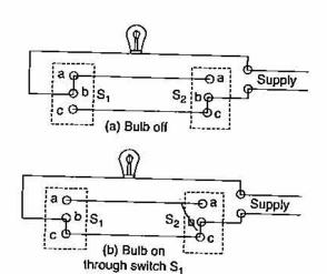
Either of switch is ON, Bulb will be ON.
