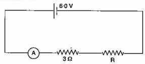
When the circuit is switched on, the ammeter reads 0.5 A.
